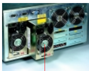
Redundant power supply
